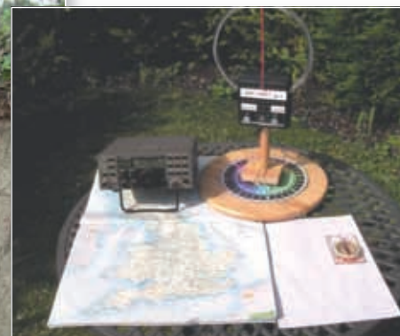
This version (above) of the Huff Duff 7 was built by Derek Brooks M0BNZ, who co-operated with Geoff G3XGC to take bearings on GB75PW.
